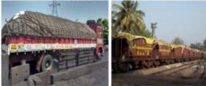
COVERING OF TRUCKS / WAGONS WITH TARPULINS
