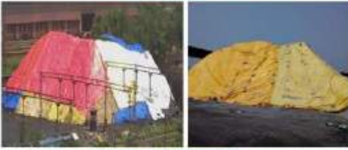
COVERING OF STACKS WITH TARPULINS
