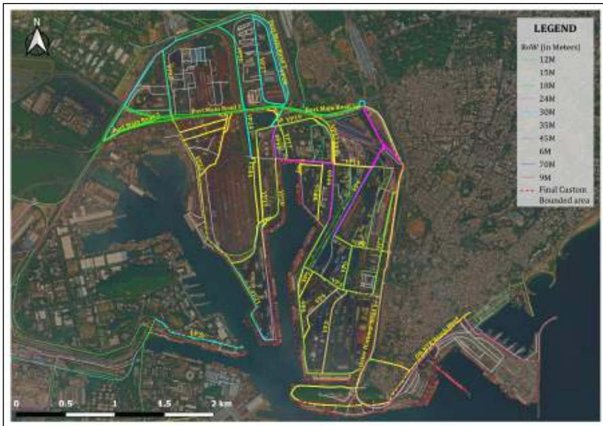
Figure 7-10: RoW details of the roads present near East and West Quay and storage areas
